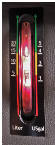
Figure 5 Fuel tank level LED lights
