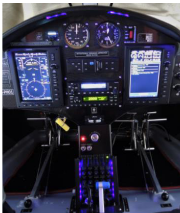
Figure 3 Glare-shield and breakers UV-LED lights
