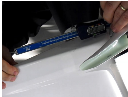
Figure 27-004 Rudder radial free play check
