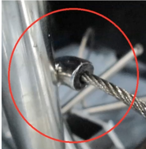
Figure 27-002 Upper pedal-rudder cable joint
