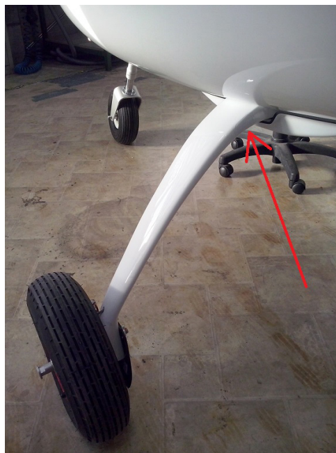
Figure 32-004 MLG access patch location
