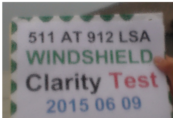
Figure 56-003 Example of inadequate window clarity
