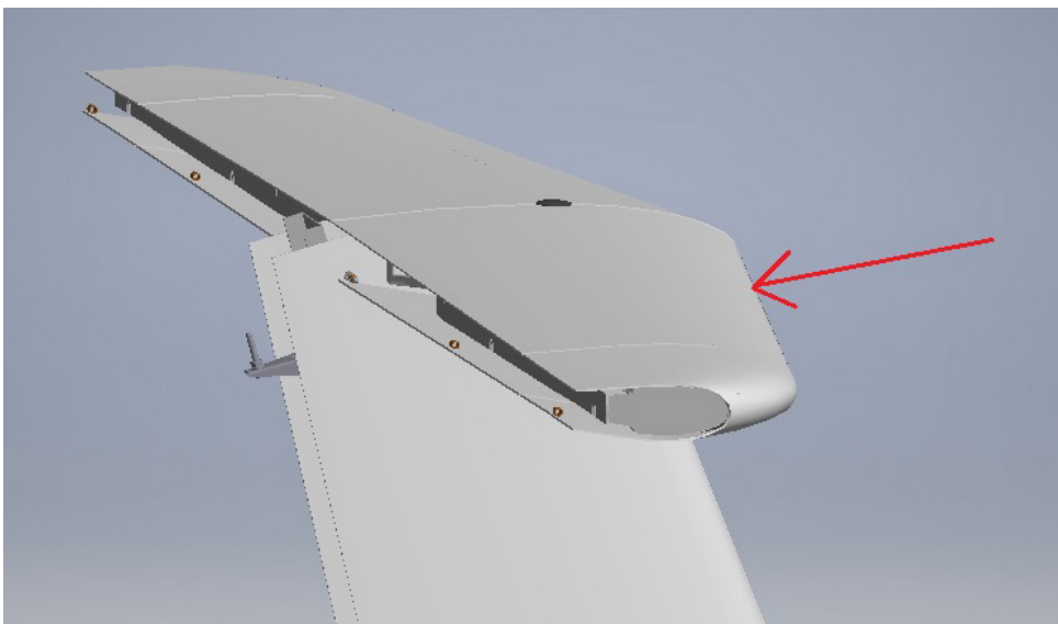
Figure 51-004 Horizontal stabilizer leading edge bonding line
