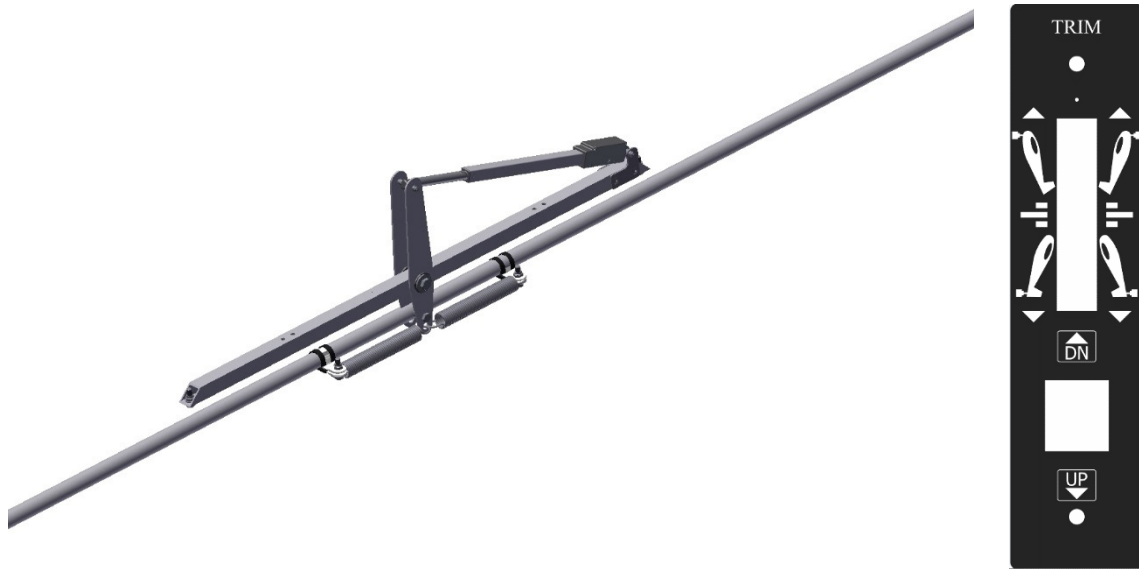
Figure 27-007 Elevator trim system and cockpit switch/display
