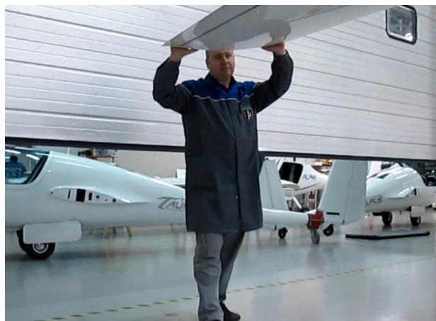
Figure 07-001 Lifting the wing
