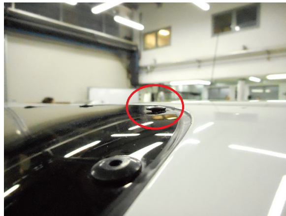
Figure 56-004 Example of loosened window rivet
