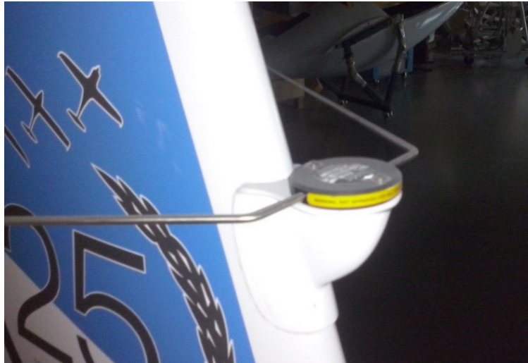
Figure 34-010 NAV antenna installation
