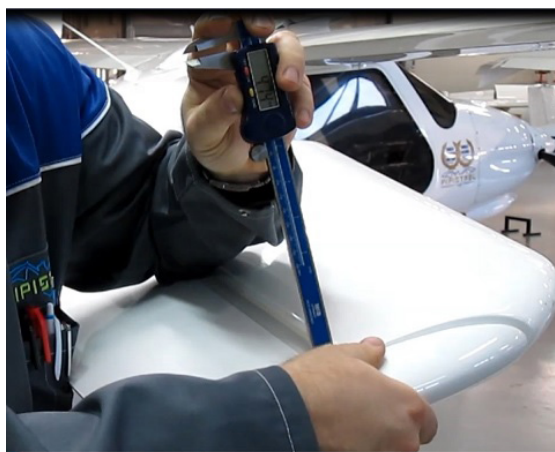
Figure 27-009 Elevator radial free play check
