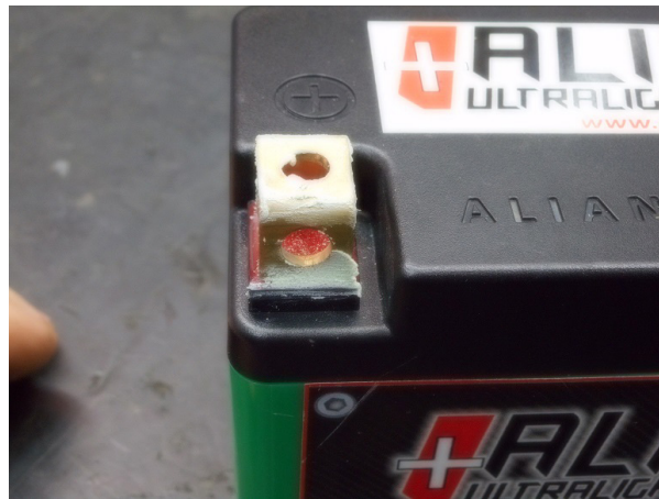
Figure 24-002 Example of battery terminal oxidation
