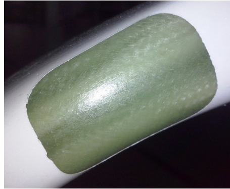
Figure 32-006 Example of a MLG in very bad condition (severe internal whitening)
