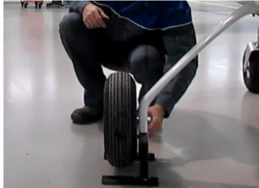
Figure 07-002 Landing gear stand placement
