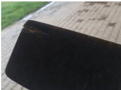
Figure 61-002 Example of cracked propeller blade
