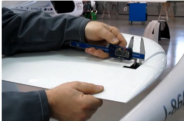
Figure 27-008 Elevator axial free play check
