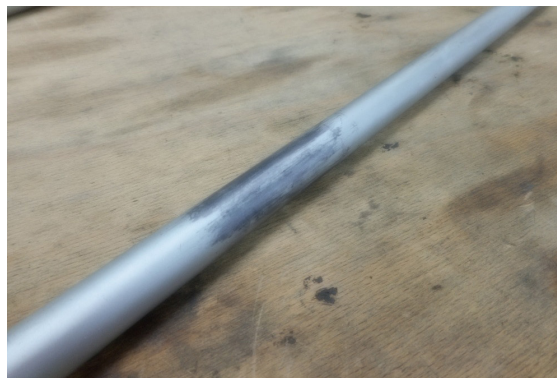
Figure 27-010 Horizontal elevator pushrod surface discoloration
