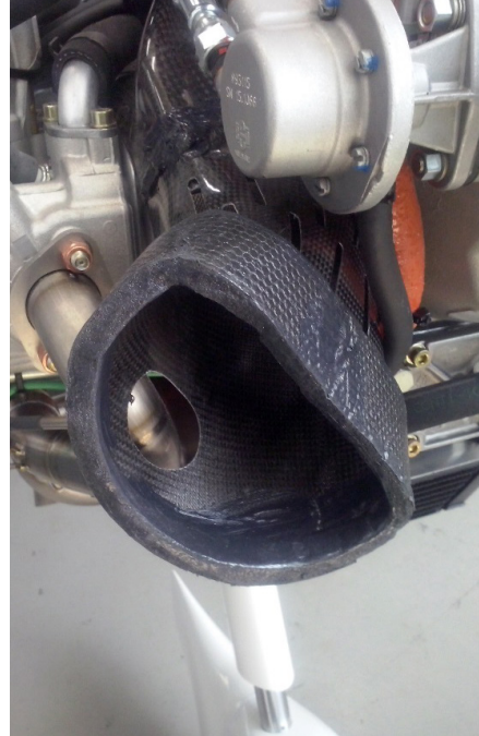
Figure 71-003 Ram cooling air intake
