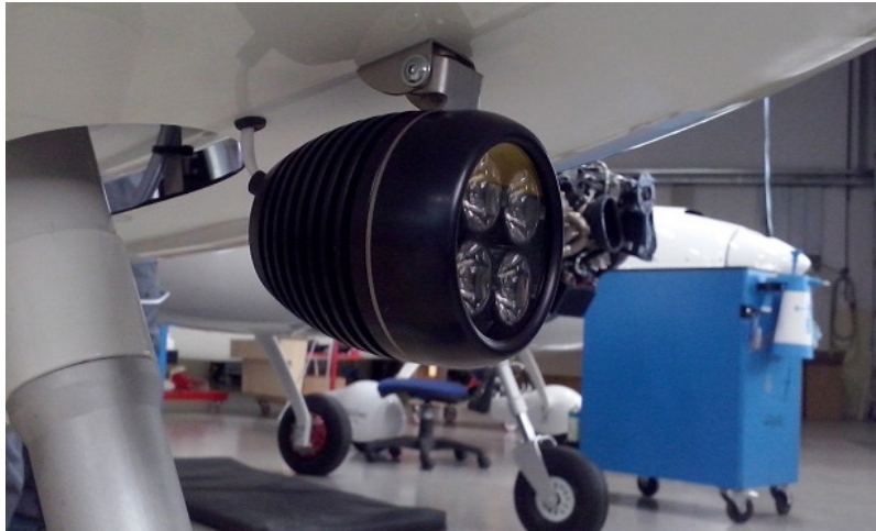
Figure 33-002 Landing light installation
