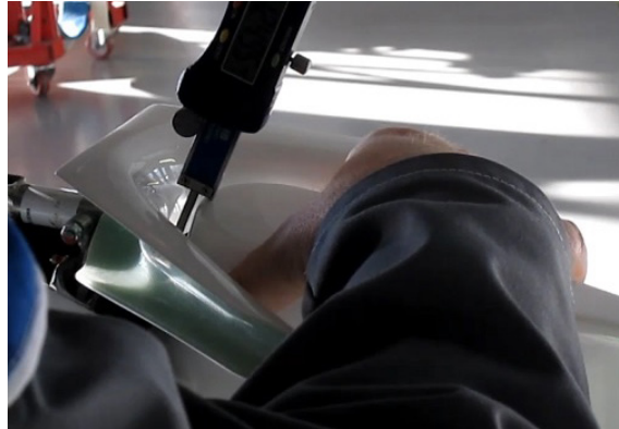
Figure 27-005 Rudder axial free play check
