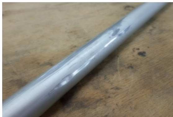
Figure 27-011 Horizontal elevator pushrod surface gouges
