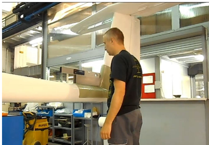
Figure 08-001 Leveling tool and spirit level setup
