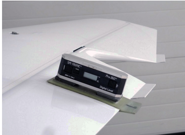
Figure 27-0016 Elevator deflection angle adjustment
