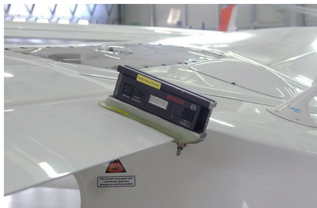
Figure 27-0017 Flaperon deflection angle adjustment
