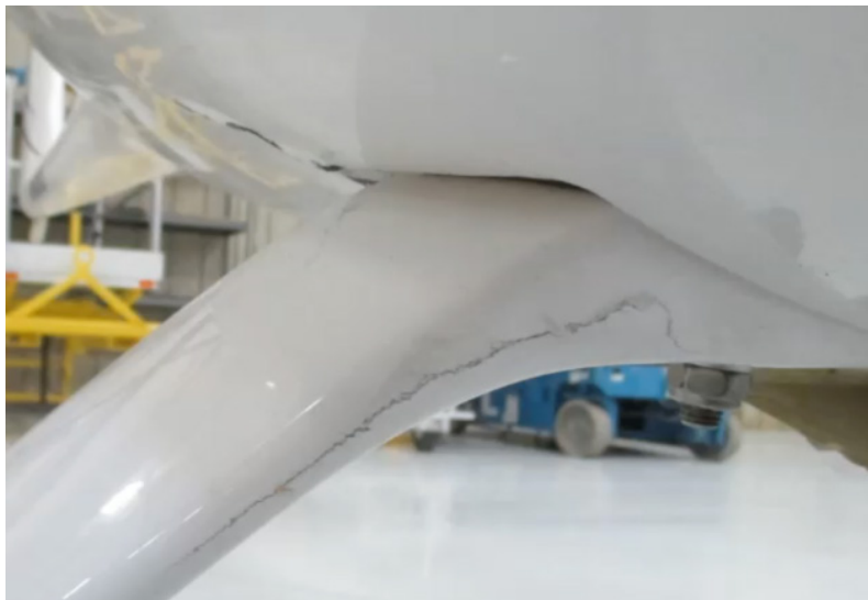
Figure 32-003 Example of a damaged main landing gear strut
