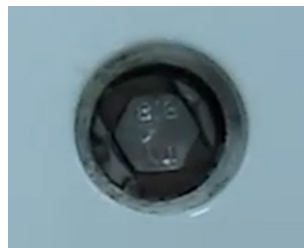
Figure 55-002 Attachment bolt assembly head orientation
