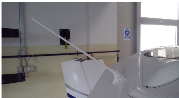
Figure 34-008 COM antenna installation
