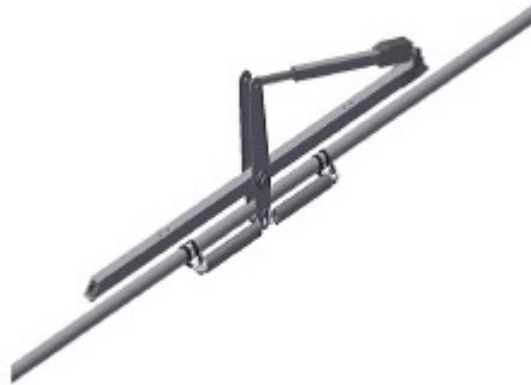
Figure 22-003 Elevator Trim Installation
