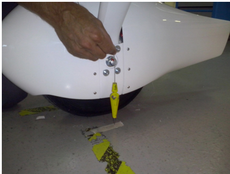
Figure 08-003 Plum bob from center of the MLG wheels
