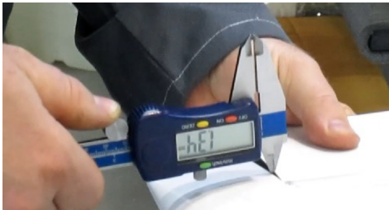
Figure 27-014 Flaperon axial free play check
